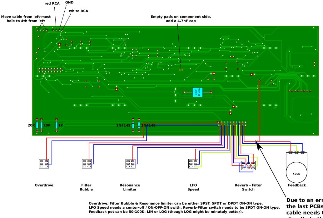
× Denotes cut trace, only cut the trace that goes IN BETWEEN the two pads.
